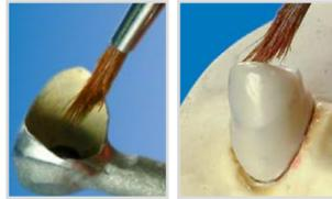
**Attachment glue:** to glue the Usig friction-generating coping in the tertiary part. There has to be a slot (0.2 mm) for the glue. This slot guarantees a tension-free fit and will be filled by the glue.
