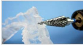
**2.** Grind the borders with the tungsten carbide bur (> 20 000 rev/min). Smooth the borders, ...
