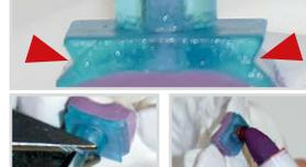
**12.** Marked areas have to be free of Erkogum. Now mark the outermost surface of each spacer with an appropriate pen.
