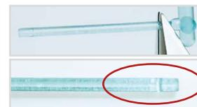
**4.** Cut off the spacer holding pins.
