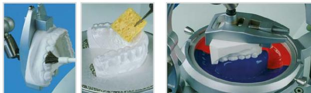
**28.** After cooling down open the Occluform and take out the model together with the model pot.
