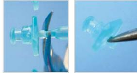
**8.** Cut the anchors as shown on the picture.
