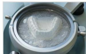
**2.** Always thermoform the plate together with the ex works applied insulating foil and allow to cool down.
