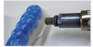
**5.** Erkoloc-pro can be shined with the hot air burner (177 540), thereby only work on the model and do not heat the holes for the anchors (risk of deformation).
