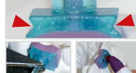
12. Marked areas have to be free of Erkogum. Cut all pins. Now mark the outermost surface of each spacer with an appropriate pen.
