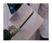
3. Allow heat gun to warm up and pass over joint 3 times or until surface is glossy.
