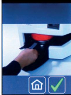
to 6 + 7. After the cooling time the display shows the further steps to pull the model pot out of the unit and remove model and foil out of the foil reception (g - i).
