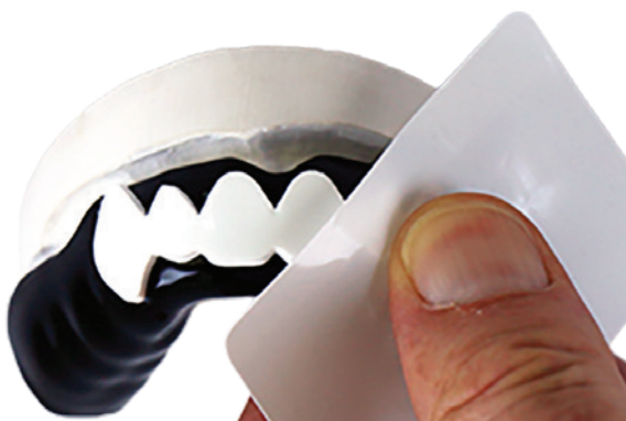
Step 3. With the hot air pen, heat each tooth (only a small amount of heat is required, 3-4 seconds) and then using an FG Sheet (art # 177400) press to shape onto the mouthguard. Work from one side of the tooth section to the other to allow the previously heated area to cool slightly to avoid distorting the work you have done.
