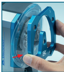
15. The model moves to the demoulding frame.
