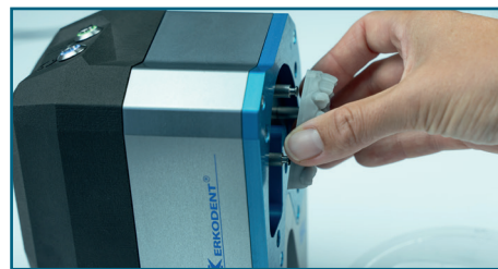
12. Unmount the model upwards. The device is ready for the next separation process.
